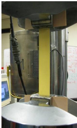
Figure 6. Sample held in the grips with card stock to prevent jaw breakage.
