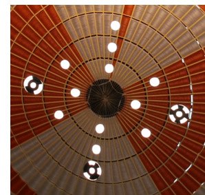
Figure 2. Retro-reflective target pattern on each test article.
