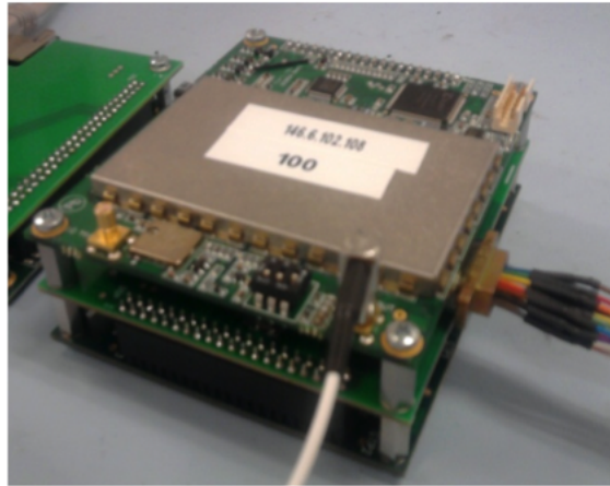
Figure 2. FOTON GNSS Receiver. FOTON will be miniaturized into the PC-104 form factor for integration on CuSPED.
