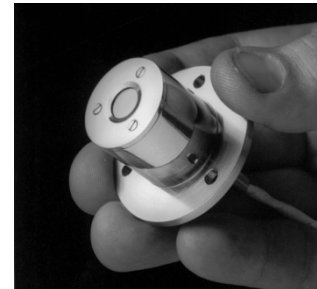
Figure 17. MEDTHERM 64 Series Heat Flux Sensor (1) (Ref. 14).
