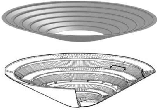
Fig. 9. Illustration of representative notional RDD design (top) in comparison to the Viking aeroshell design (bottom). 27
