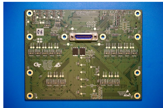
Figure 14: Top of Controller with Circular Pogo Pin Landing Pad Test Points
