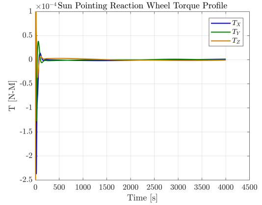
Figure 38: Sun Pointing Reaction Wheel Angular Torque
