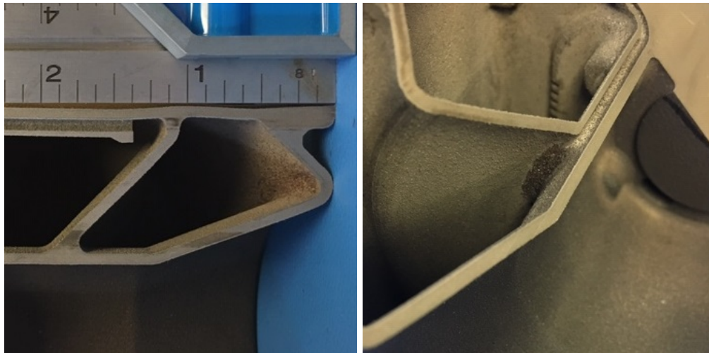
Figure 17: Examples of part abnormalities during DMLS printing. At left is an example of warping through a wall intended to be completely flat. At right is an example of residual powder fused into thick convex features, where the dark coloring and increased surface roughness in the corner indicates this phenomenon.
