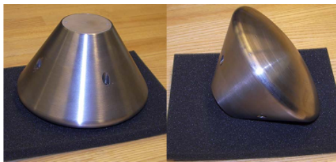
Figure 6. CEV model (PTM2) used in the pressure-telemetry tests. 33
