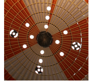
Figure 2. Retro-reflective target pattern on each test article.
