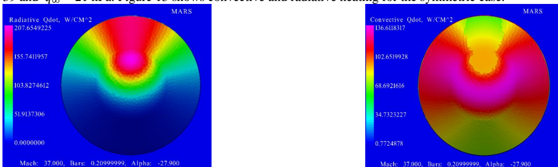
Figure 13. Radiative and convective heating for the symmetric HIAD.
