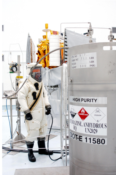
Fig. 2 A technician loads hydrazine onto the MESSENGER spacecraft, Credit: NASA/Johns Hopkins APL
