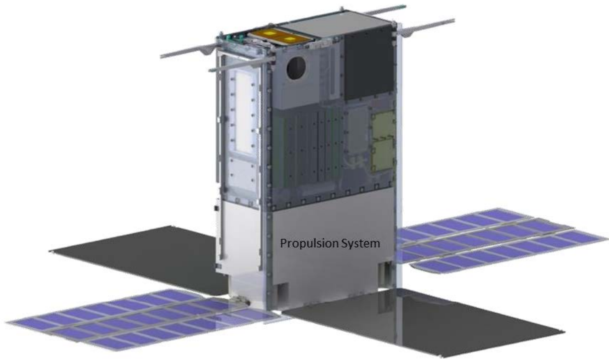
Fig. 6 Lunar Flashlight spacecraft, specifying the location of the propulsion system
