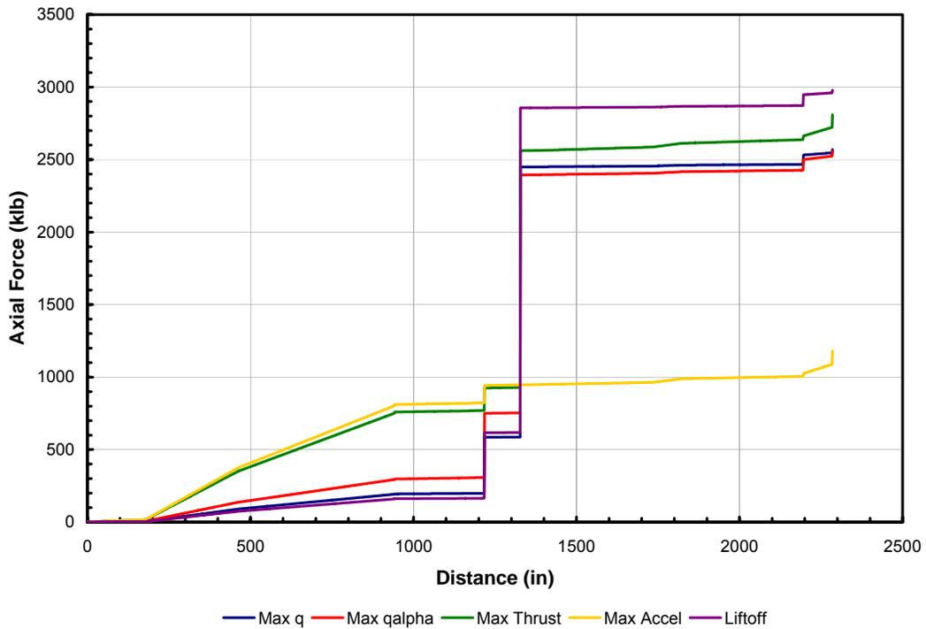
Figure 27. Axial Force Magnitude Variation along the Fuselage for each Load Condition of the EELV
