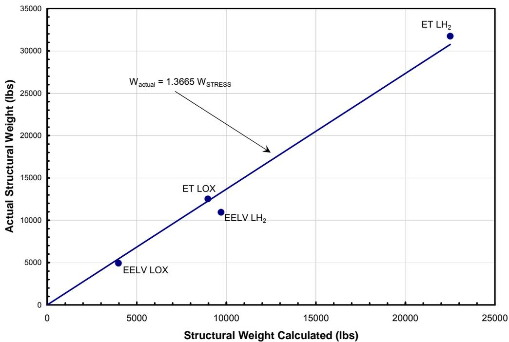
Figure 21. Linear Regression of Structural Weight.
