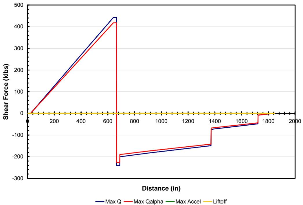
Figure 31. Shear Force Variation along the Fuselage for each Load Condition of the ET
