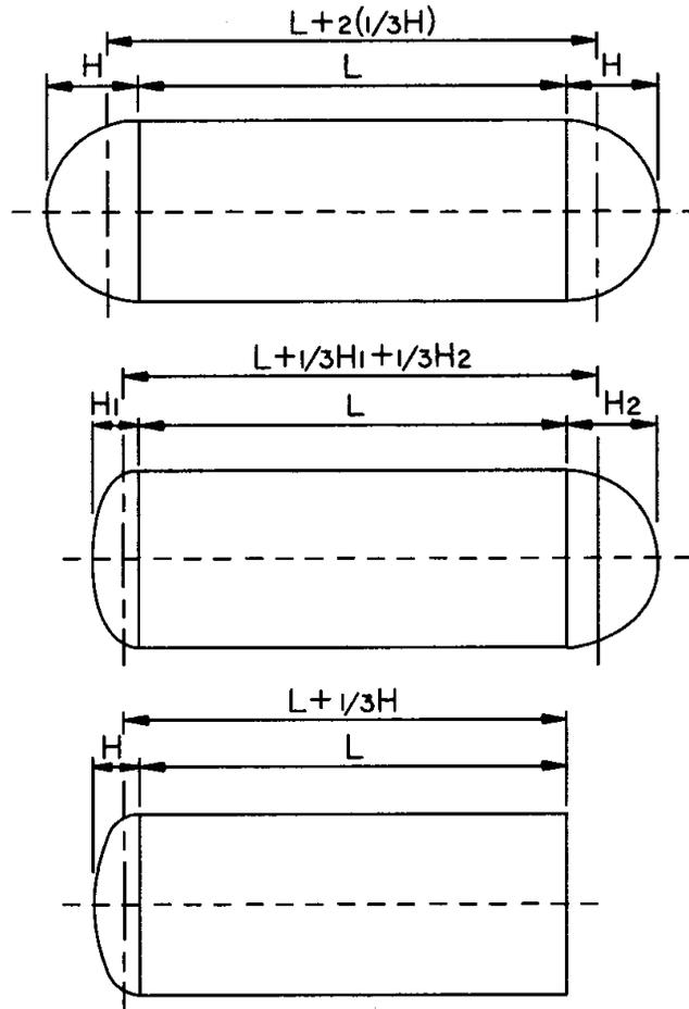
Figure 3. Effective Length of Cylindrical Tanks with Various End Closures (Jawad, *Design of Plate & Shell Structures*, p. 376).
