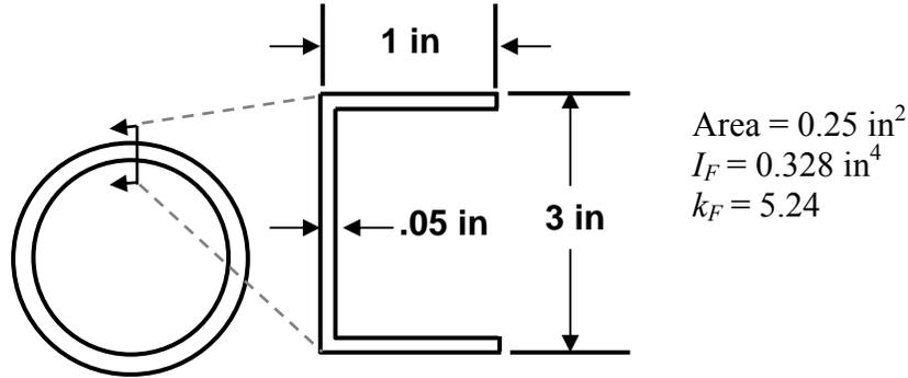
Figure 12. Shape and Dimensions of Frame Cross Section.
