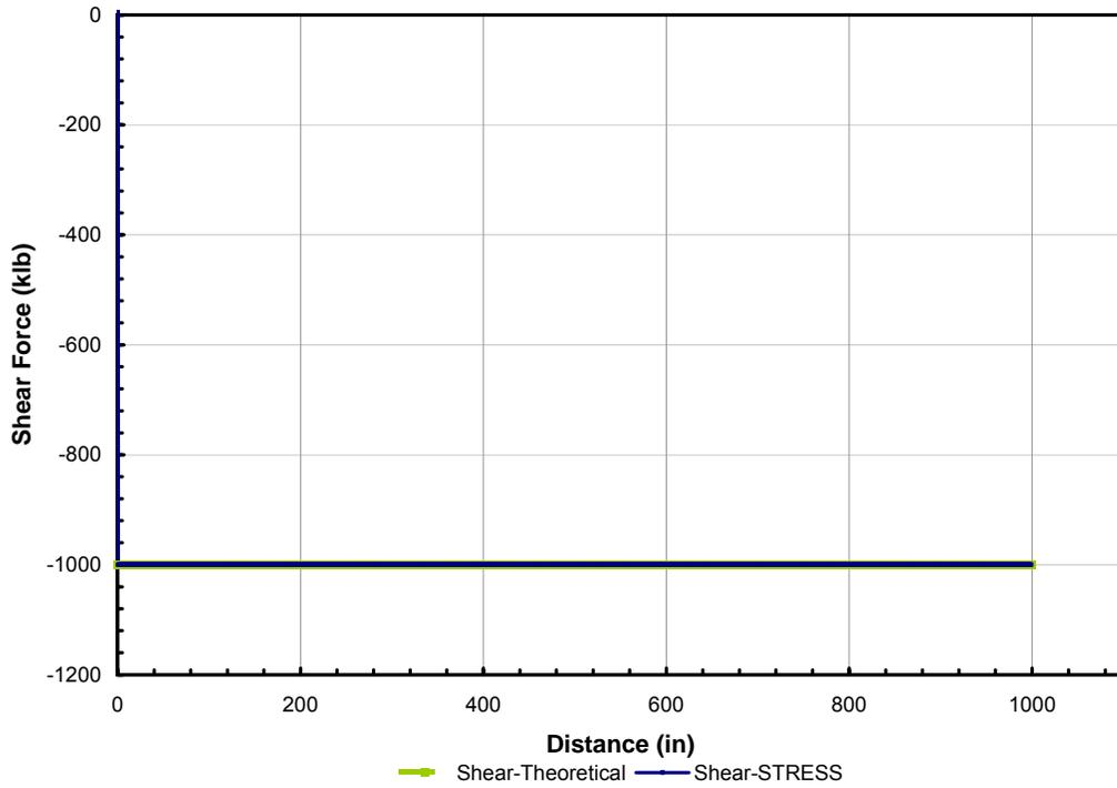
Figure 4. Shear Force Accuracy of Discretized vs. Theoretical Method for End Loaded Cantilevered Beam
