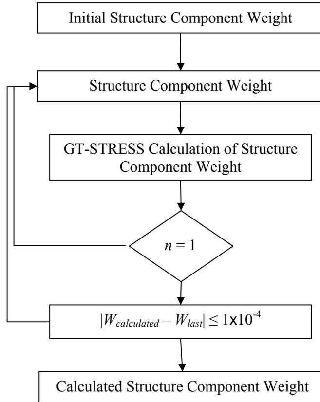
Figure 13. Convergence Process for Determining Structure Component Weight.
