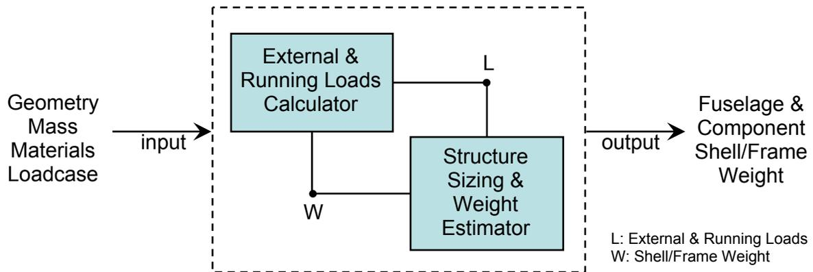
Figure 14. MDA Model of GT-STRESS Program Operation.
