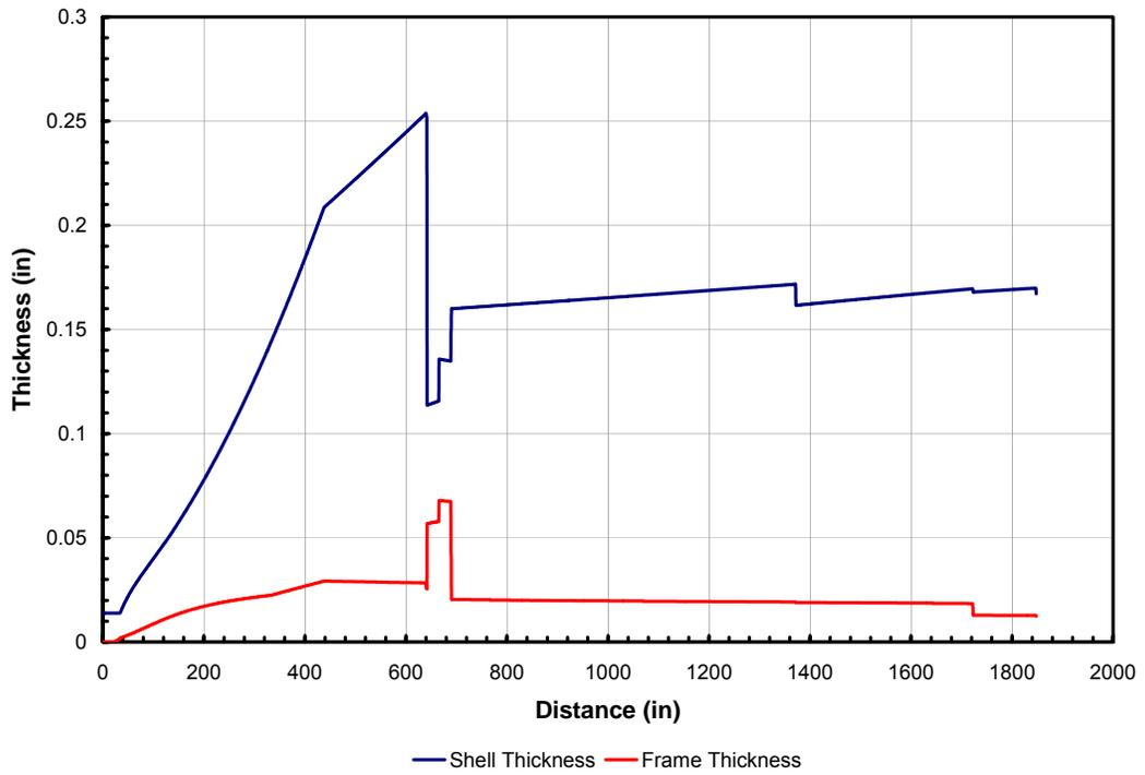
Figure 20. Shell and Frame Thickness Variation along the ET.
