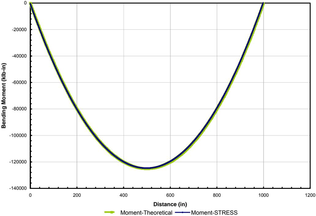
Figure 6. Bending Moment Accuracy of Discretized vs. Theoretical Method for Uniformly Loaded Simple Support Beam
