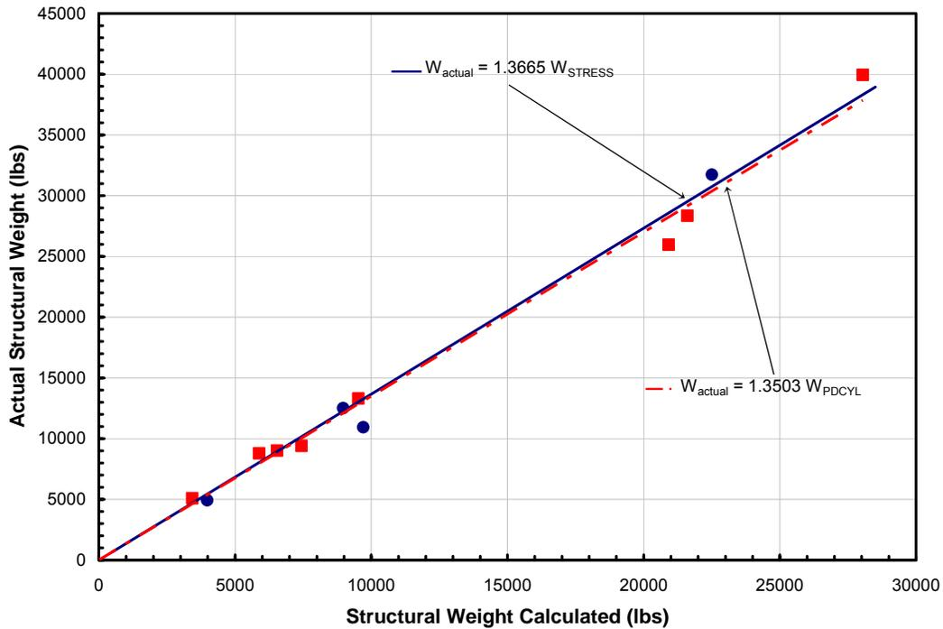
Figure 23. Regression Comparison of Structural Weight Results from GT-STRESS and PDCYL.
