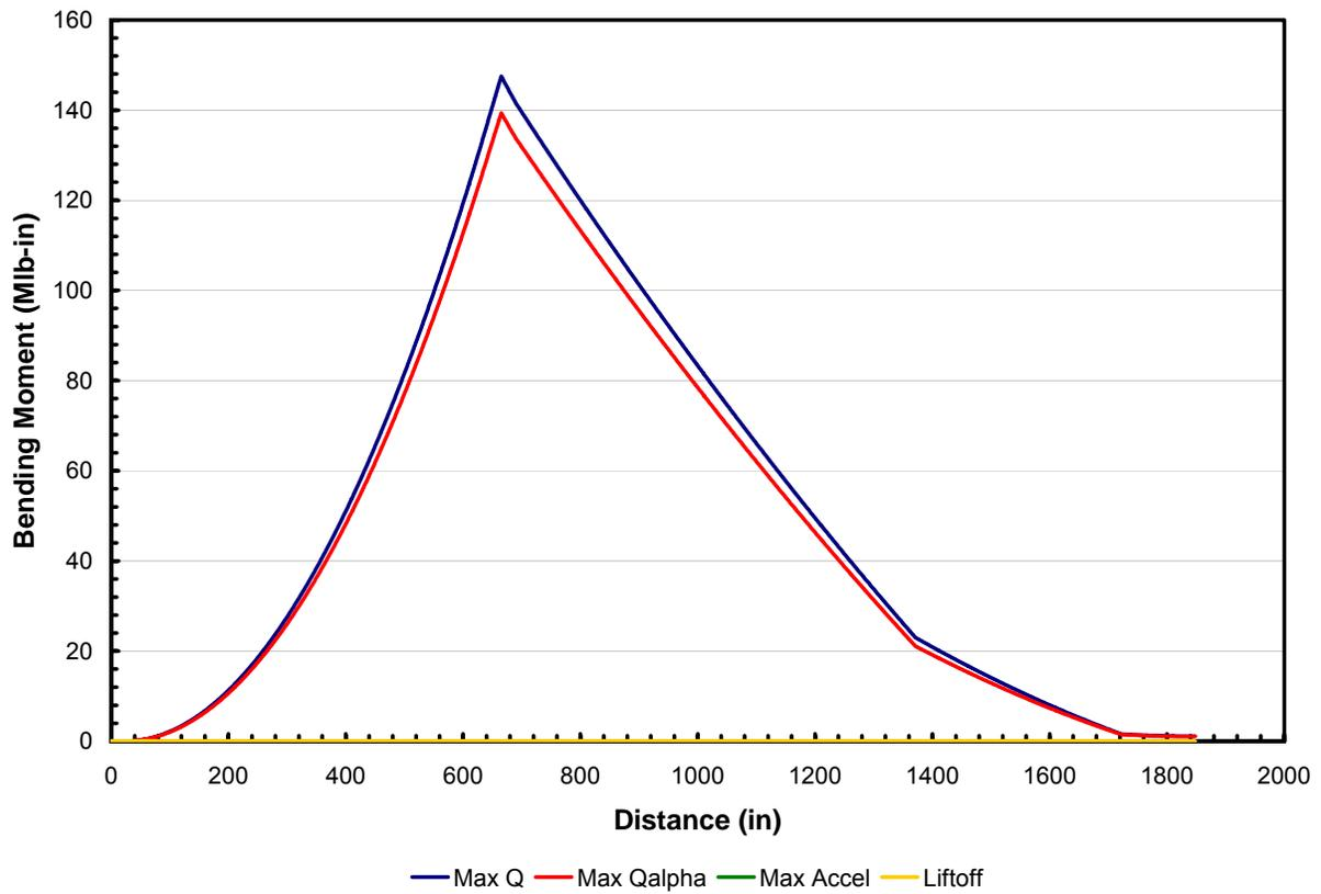
Figure 32. Bending Moment Variation along the Fuselage for each Load Condition of the ET
