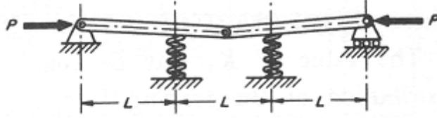
Figure 11. Model for General Instability Failure
