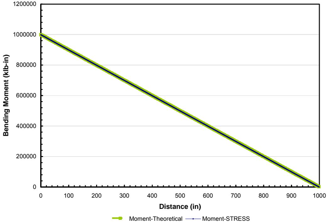
Figure 7. Bending Moment Accuracy of Discretized vs. Theoretical Method for End Loaded Cantilevered Beam
