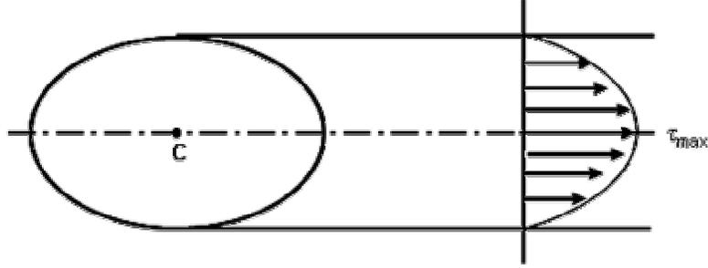
Figure 9. Shear Stress Distribution over an Elliptical Section
