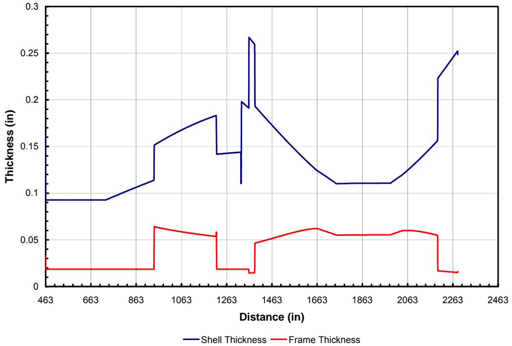
Figure 19. Fuselage Shell and Frame Thickness Variation along the EELV.
