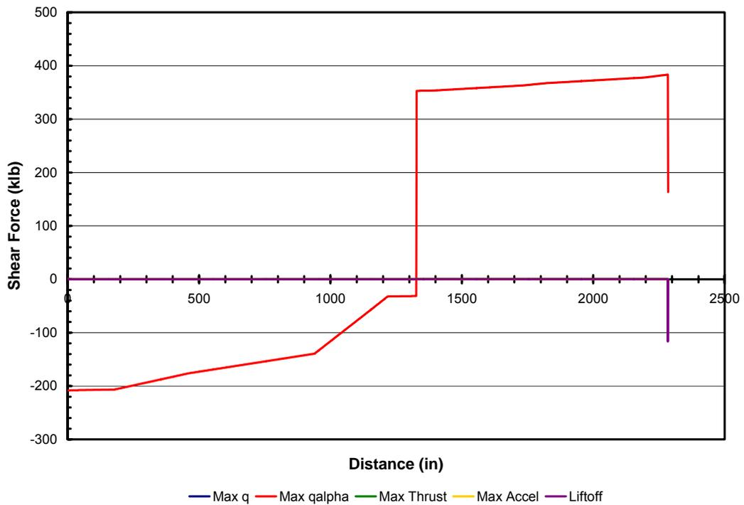
Figure 28. Shear Force Variation along the Fuselage for each Load Condition of the EELV
