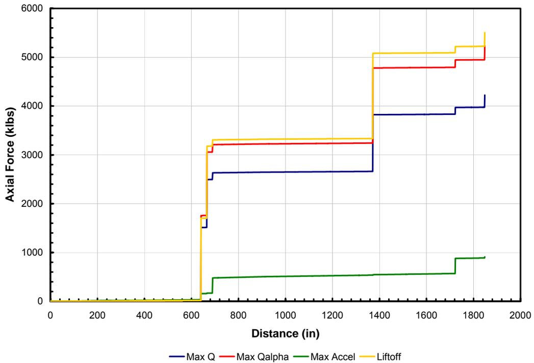
Figure 30. Axial Force Magnitude Variation along the Fuselage for each Load Condition of the ET
