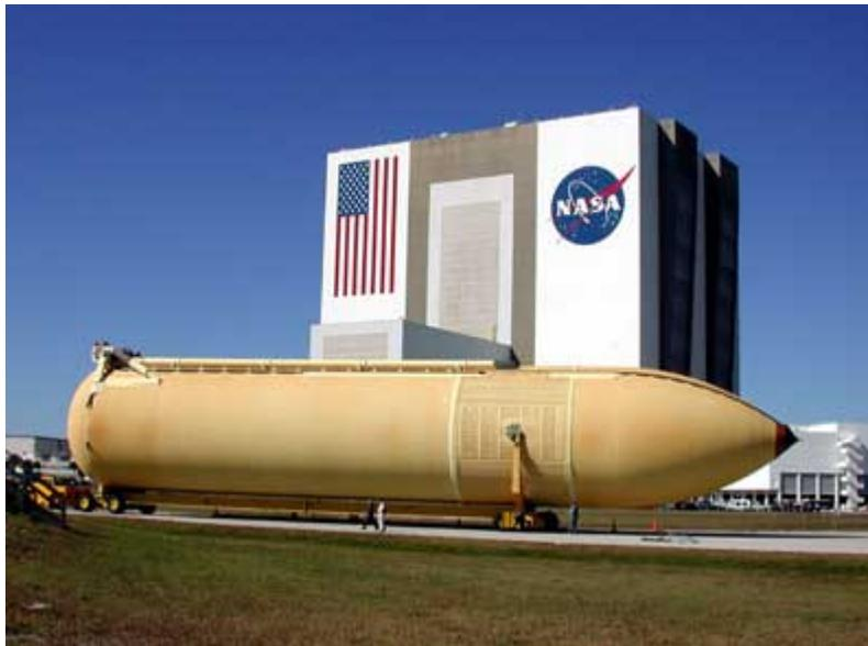
Figure 16. Space Shuttle External Tank.
