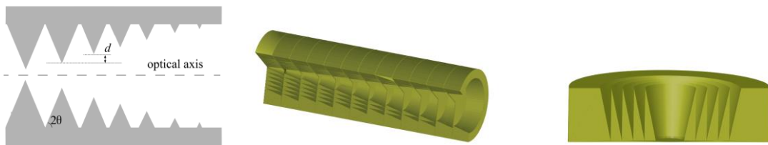
Figure 11 - (left) Sawtooth CRL (center) Assembled Stack of SPLs (right) One Element of the SPL Assembly [32]
