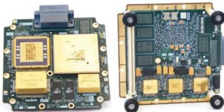
Figure 12. JPL Manx Computer Card (a) Front (b) Back (from Bolotin et al 2018).
