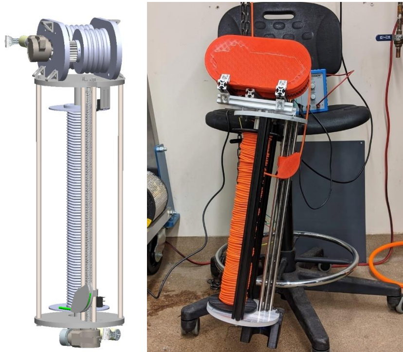
Figure 6. VERNE Tether Management System (a) CAD Model (b) Prototype (F. Bryson).
