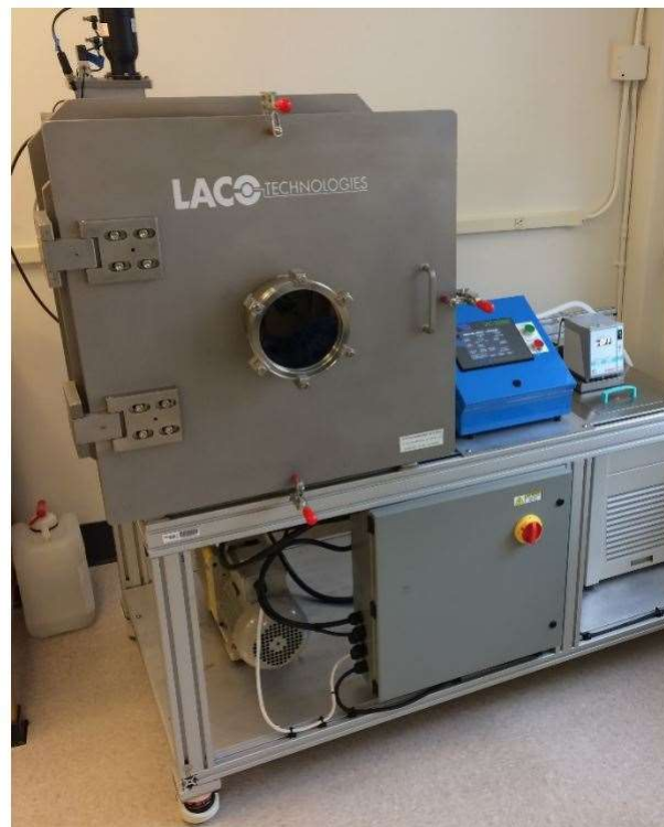
Fig. 15 SSDL Thermal Vacuum Chamber
