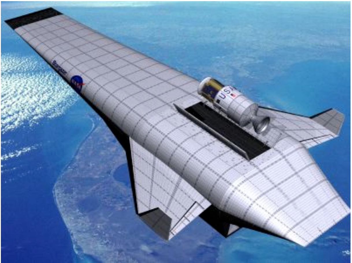
Figure 1: Stargazer vehicle in flight, deploying its upper stage.
