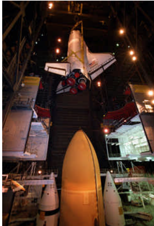
Figure 3.11: Mating of Atlantis and the STS Stack xxxii
