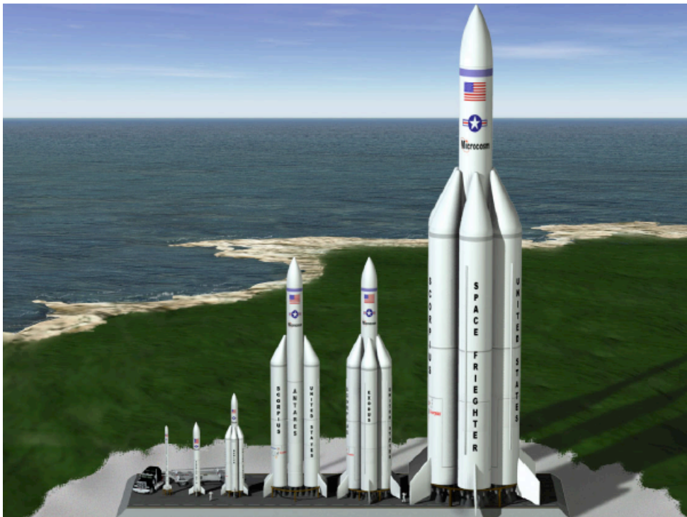
Figure 1: Microcosm Scorpius Family On the left, are the SR-S and SR-XM suborbitals and the Sprite Small Launch Vehicle. The intermediate-sized vehicles in the center are Antares and Exodus. The Heavy Lift Space Freighter is on the right. (Source: James R. Wertz, Robert Conger, Jack Kulpa, “Responsive Launch with Scorpius of Low-Cost Expandable Launch Vehicle,” Microcosm Inc, AIAA LA Section/SSTC 2003-500)
