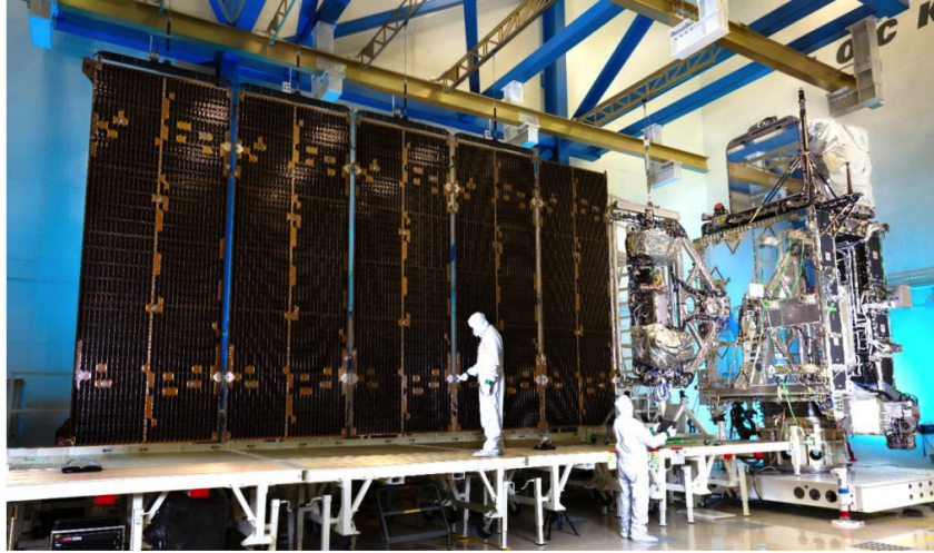
Fig. 8 GOES 16 solar array installation[24]
