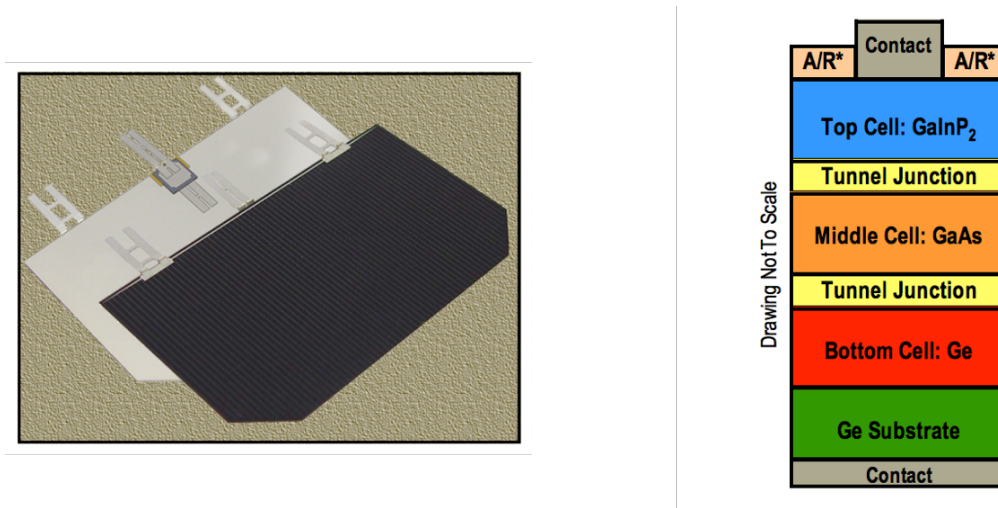
Fig. 9 Spectrolab 28.3% Ultra Triple Junction solar cell (left) and the cell structure (right)[25]
