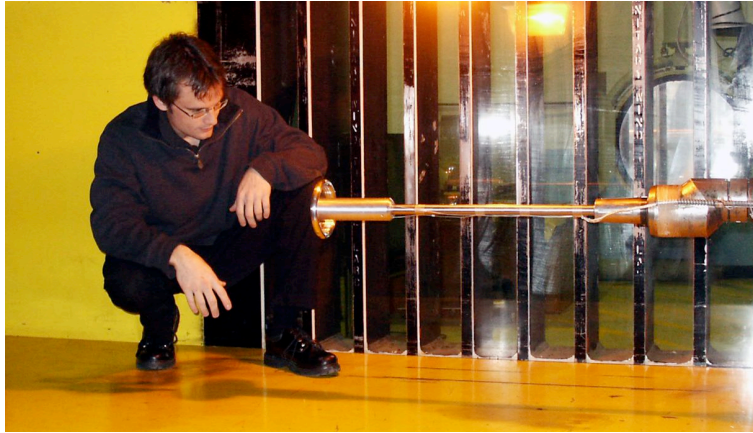
Figure 37: Tension cone model assembly within the LUPWT test section (shown with author).
