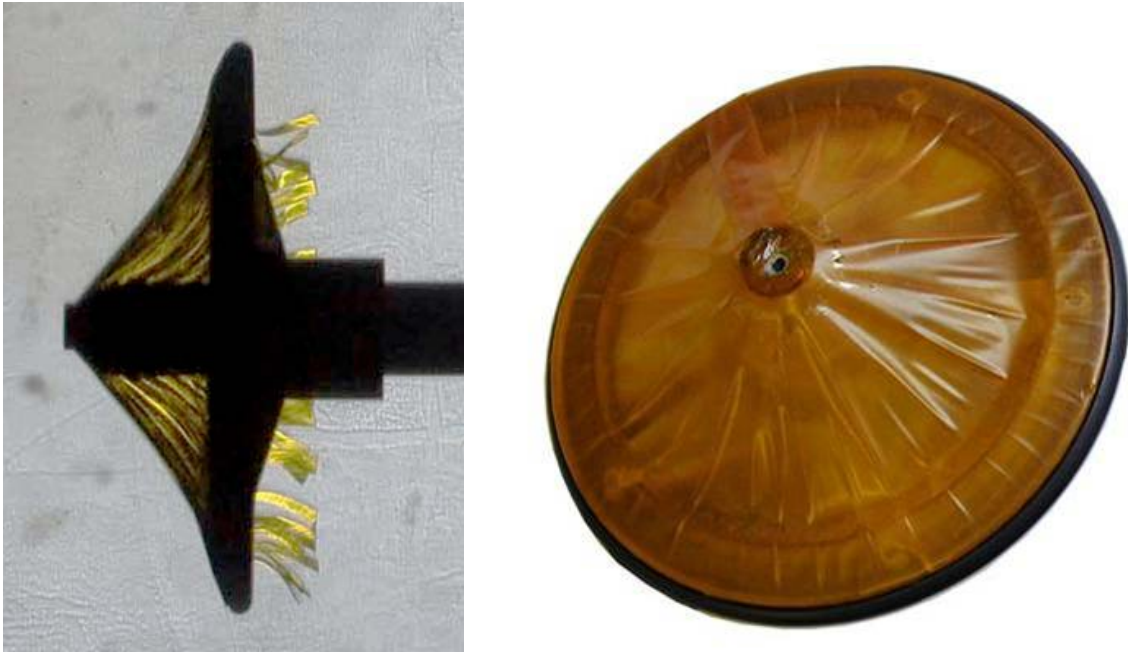
Figure 3-2: The \text{CF}_4 wind tunnel test model during testing (left) and after testing (right) [20].
