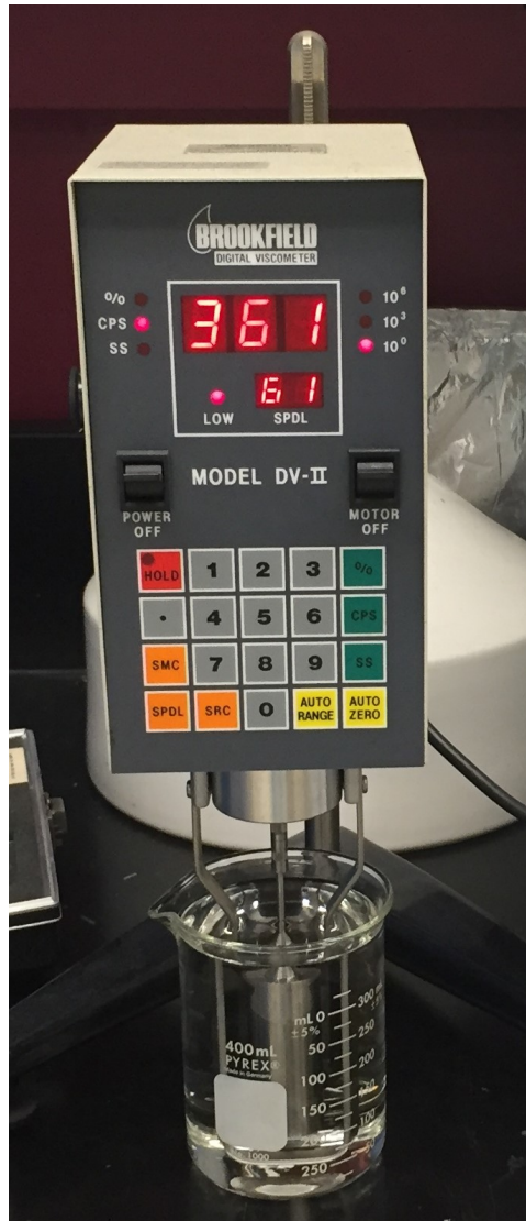
Figure A.6: Experimental set up with rotational viscometer.
