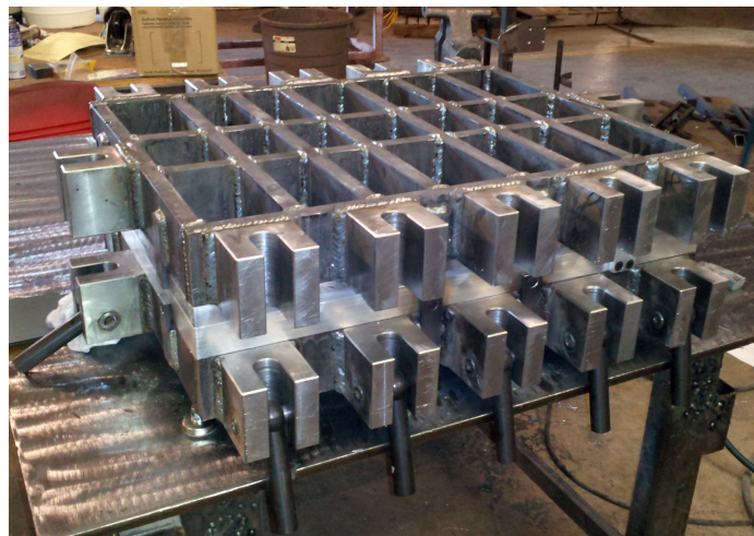
Figure 1.13: A double-sided, rigid aluminum mold for an RTM process (Credit: JHM Technologies, Inc.).
