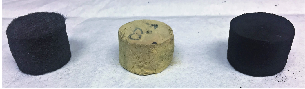
Figure 2.2: Material at each step in experimental processing (left to right): dry felt prior to processing, virgin TPS, and charred TPS.
