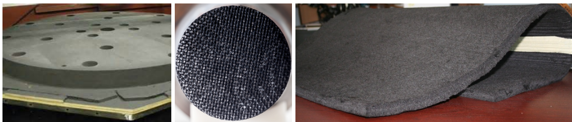
Figure 1.6: Examples of fiber substrates (left to right): FiberForm® block, woven carbon, and carbon felt (Credits: FiberMaterials, Inc., Venkatapathy and Ellerby [15], and Gasch, et al. [16]).
